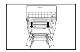
**NOTE:** The *Drum Unit* is sensitive to light. Never expose the *Drum Unit* to light for more than five minutes.
